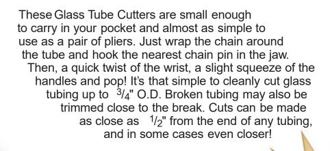
Unique cutting action based on the original Wheeler "Squeeze and Pop" cutting principle.
